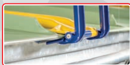
❌ Tool closes completely Seam is fully compressed
